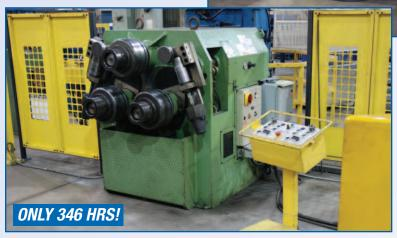
1999 **COMAC** Angle Rolls Model 307 HV3 – CA3, 12.5" Roll Diameter, Shaft Diameter 3.97", Max Capacities: Solid Flat 4"x1", Solid Rectangle 7"x1.5", Solid Square 2.5", Solid Round 3", Hollow Rectangle 4.5"x2"x5/32", Angle 4"x1/2", Channel 7"x14.75", I Beams 7"x20", W In3, 2.75", Advancement Profile Speed: Variable 0-23 FPM, 15 HP, Light Curtains, 440V, sn 307325HV3
