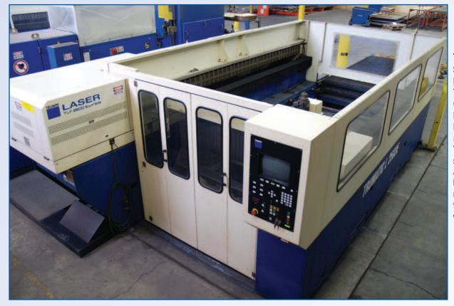
**TRUMPF** Laser Cutting System Model Trumatic L2503E, Trumatic Control, TLF 2600 Turbo Resonator, Chiller, Dust Collector, Auto Pallet Changer, Light Curtains. Laser Power 2600 W, Table 5'x10', Travels: X-61", Y-121", Z-4", 460V, 70Hz, sn 902914 **Auctioneer's Note:** Trumpf Laser was in operation until mid-January 2013, at which time the resonator stopped working.
