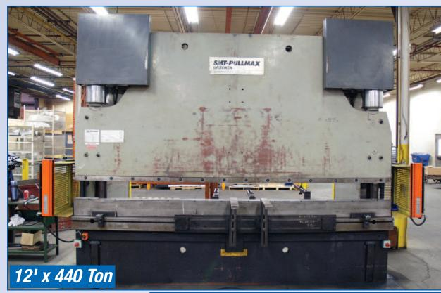
PULLMAX 12' x 440 Ton Press Brake, Model EKP M400, Overall Bed Size 146", Distance Between Housing 124", Open Height 31.5", Stroke 11.8", Throat 10-1/4", Tool Space 23.6", Speed 21 IPM, Guard Distance 4.3", Stop Time 1 ms, Lab-A-Tron DX-124DC Swing Open Light Curtains Front & Back, 550V, 28 HP, sn 3089
