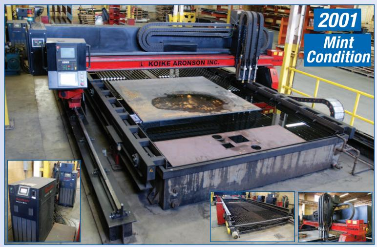
**KOIKE ARONSON** Plasma Cutting System, Model VGM 2500, Versagraph Millenium Series, Dual 11'x24' Tables, Quick Panel Total Touch Control, 2 Torch Heads, 1 Etching Head, 2 Hypertherm HyDefinition (HD) 4070 Plasma Cutters Plus Gas Consoles (sn's 4070-000155 & 600), Cutting Width 100", Cutting Length 178" Expandable, Internal Width Between Heat Shields 176", Rail Gauge 189", Total Width 235", Rapid Traverse 800 IPM, Contour Speed 400 IPM, 10 Tools, 11'x21' Pallet Changer, Notching, sn VGM3501
